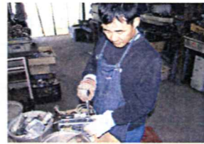
Recycling by disassembling gas pots
